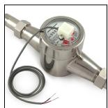
Flow sensors with 3 wires and runs on 5V can also be used with OpenSprinkler. In this case, insert the ground wire (typically black colored) GND, 5V wire (typically red colored) to VIN, and the sensor wire (typically yellow) to SN1.
