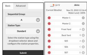
• Remote Station (IP): This allows one OpenSprinkler to command a different OpenSprinkler. The remote station is identified by its IP address, port number, and station index. For example, Zone 1 on the master controller can be mapped to Zone 5 on the remote controller. Both controllers must use the same device password (thus eliminating the need to specify the remote controller's password separately).
